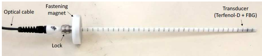
Fig. 1.12. Photograph of an FBG sensor. The dark spot on the right extremity is the Terfenol-D tube (Fracarolli et al., 2016)
