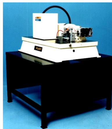
Fig. 2. Universal machine for HFFR test
