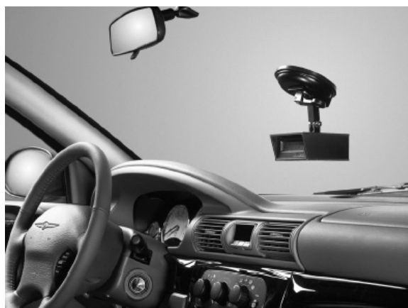
Fig. 1. The portable decelerometer XL Meter Pro Beta, arranged in the working position
