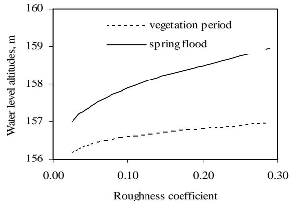
**Fig. 4.** Water level altitudes in the Nemėža stream, when the average spring flood and vegetation period discharge is with 10 % probability at varied roughness coefficient
