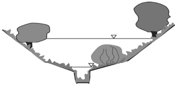
**Fig. 5.** Water levels in modelled profile, when spring flood discharge is with 10 % probability and the average discharge of vegetation period is with 10 % probability as well (roughness coefficient  $n = 0.080$ )
