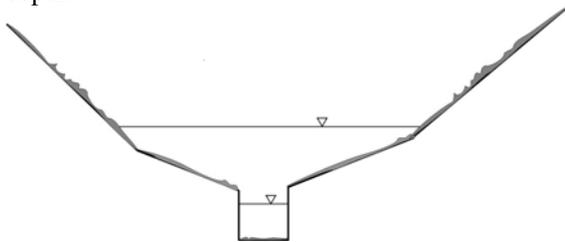
**Fig. 3.** Water levels in modelled profile, when spring flood discharge is with 10 % probability and the average discharge of vegetation period is with 10 % probability as well (roughness coefficient  $n = 0.030$ )
