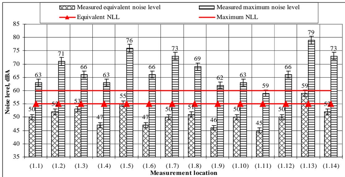
Fig 5. Equivalent and maximum noise levels in Trakai at night
