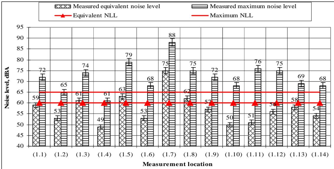
Fig 4. Equivalent and maximum noise levels in Trakai in the evening
