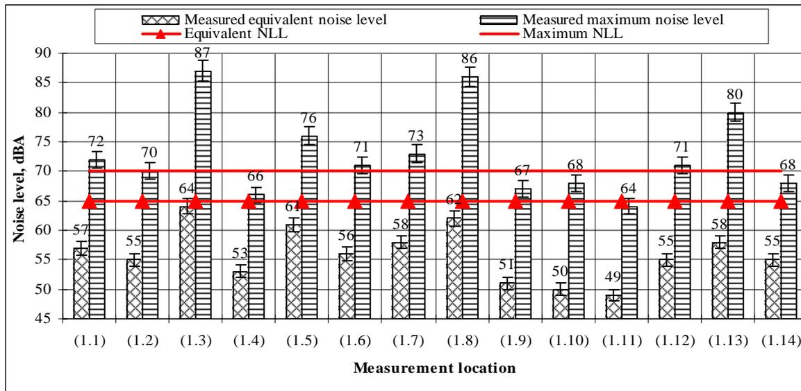
Fig 3. Equivalent and maximum noise levels in Trakai in the day time
