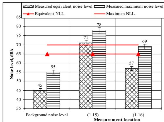
Fig 6. Equivalent and maximum noise levels at measurement locations 1.15 – 1.16 in the day time
