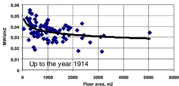
**Fig. 8** Specific heat consumption in old buildings
