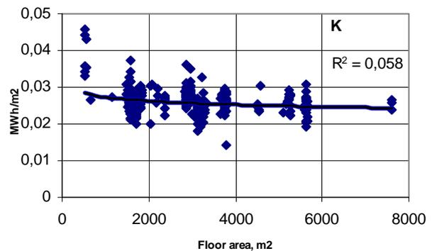
**Fig. 10** Specific heat consumption in the circuit K
