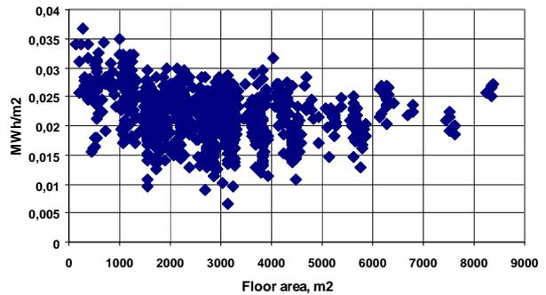
**Fig. 9** Specific heat consumption in the circuits L, K, V, Z, J in February
