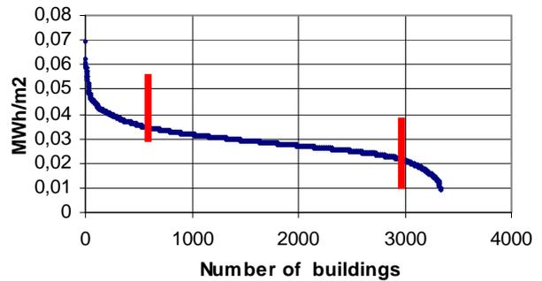
Fig. 4 Specific heat consumption in February versus number of buildings
