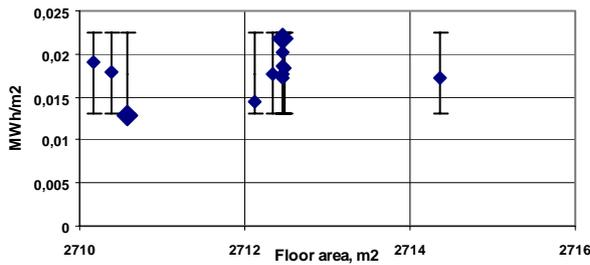
Fig. 11 Specific heat consumption in 2713 m<sup>2</sup> sister-buildings
