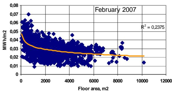
Fig. 3 Specific heat consumption in February versus building floor area
