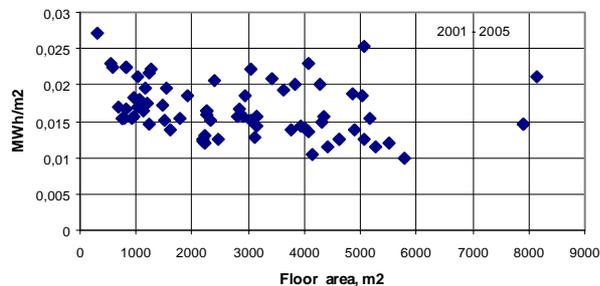
Fig. 13 New buildings specific heat consumption versus floor area
