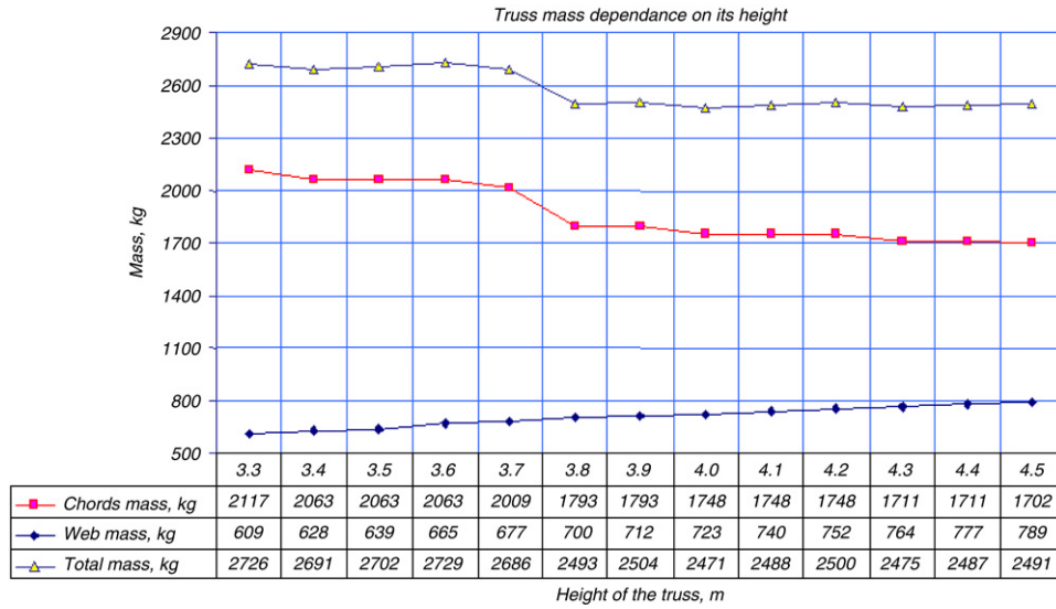
Fig. 10. Investigations results of the optimal web truss height.
