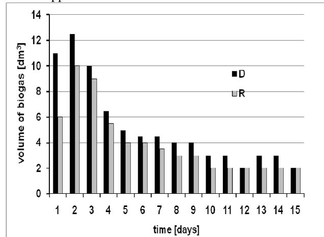
**Fig 5.** The volume of biogas generated during anaerobic digestion process (reactor D – sludge after disintegration, reactor R- raw sludge)
