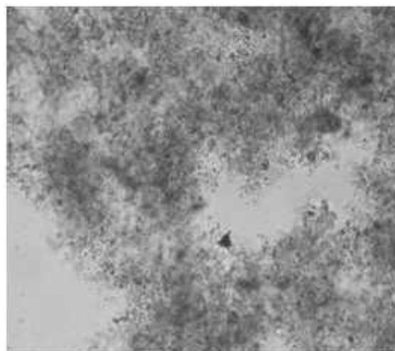
**Fig 2.** Activated sludge after ultrasonic disintegration
