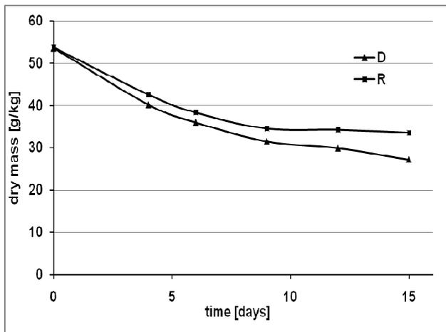
**Fig 4.** Changes of dry mass content during anaerobic digestion process (reactor D – sludge after disintegration, reactor R- raw sludge)
