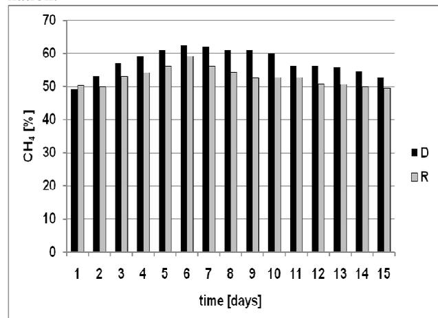
**Fig 6.** The volume of methane generated during anaerobic digestion process (reactor D – sludge after disintegration, reactor R- raw sludge)
