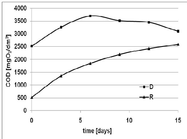
**Fig 3.** Changes of COD in supernatant during anaerobic digestion process (reactor D – sludge after disintegration, reactor R- raw sludge)
