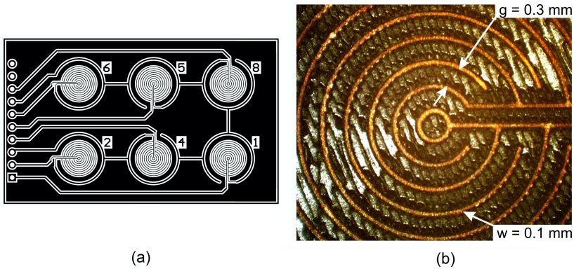
Fig. 2.33. Microelectrodes structure, where a) the resultant chip with electrodes; b) the photograph of interdigitated laser etched microelectrodes on FR-4 epoxy laminate (Novickij et al. 2015b)
