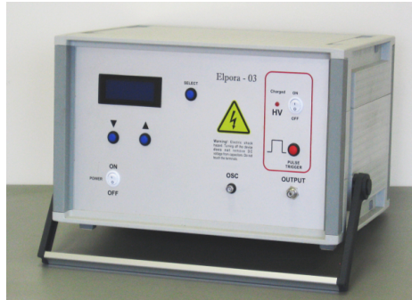
Fig. 2.25. Photograph of the nano-microsecond pulse generator prototype (Novickij et al. 2014b)
