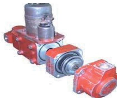
Fig 2. Piston suction pump driven by electromotor
